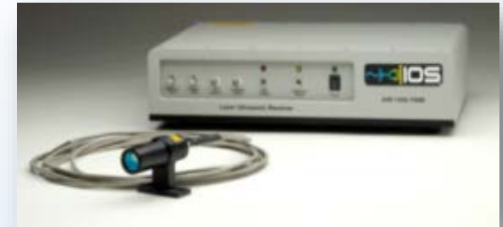
Laser Ultrasonic Noncontact Structural Inspection
